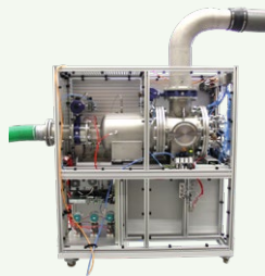
Secondary standards for flow with sonic nozzles or gas meter
