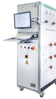
Media conditioning: pressure / humidity / temperature
